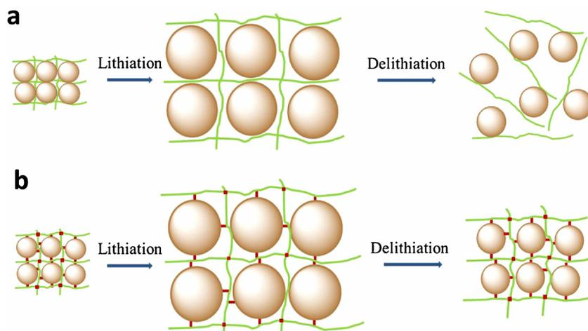
Fig. 4. The possible physical evolution in the lithiation/delithiation process for conventional electrodes (a) and electrodes with APTES (b). The particle break is not in consideration.
