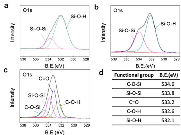
Fig. 3. High-resolution XPS spectra of O 1s regions of Si (a), Si@APTES (b) and electrode with 1% APTES (c), and the Binding Energy Assignments (d).
