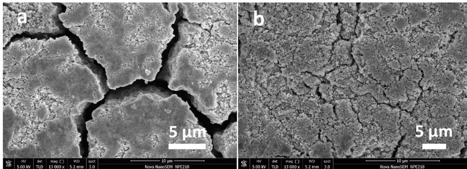
**Fig. 7.** SEM images of conventional electrode (a, b) and electrode with 0.1% APTES (c, d) after 200 cycles at 1.5 A g<sup>-1</sup>.
