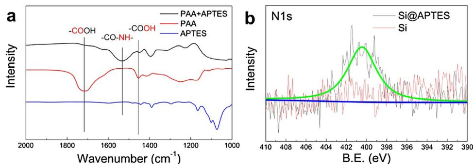
Fig. 2. (a) FTIR spectra of PAA, APTES and PAA + APTES. (b) High-resolution XPS spectra of N 1s regions of Si and Si@APTES.
