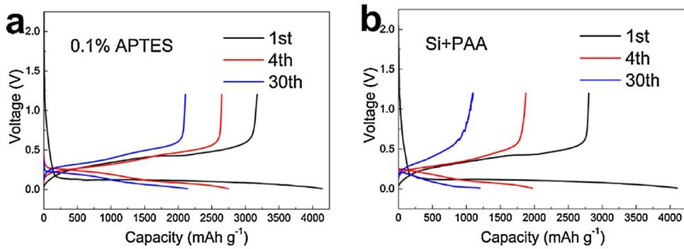
**Fig. 6.** The charge and discharge curves of electrode with 0.1% APTES (a) and conventional Si+PAA electrode (b) with 2.0~2.1 mg cm<sup>-2</sup> material loading.
