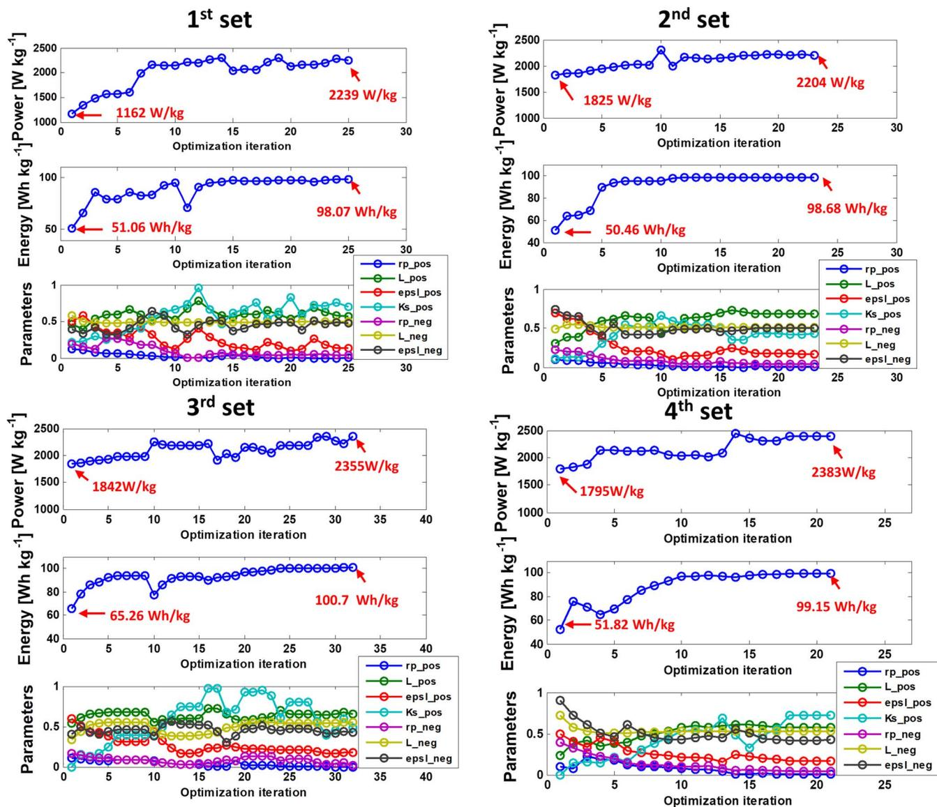
**Figure 3.** Energy density optimization with given power density requirement. The four sets show the evolution of power density, energy density, and design parameters with optimization iteration starting from different initial parameter values.
