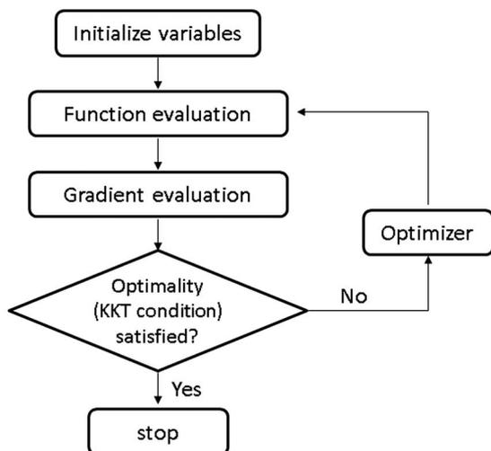
Figure 2. Flowchart of the gradient based optimization scheme.
