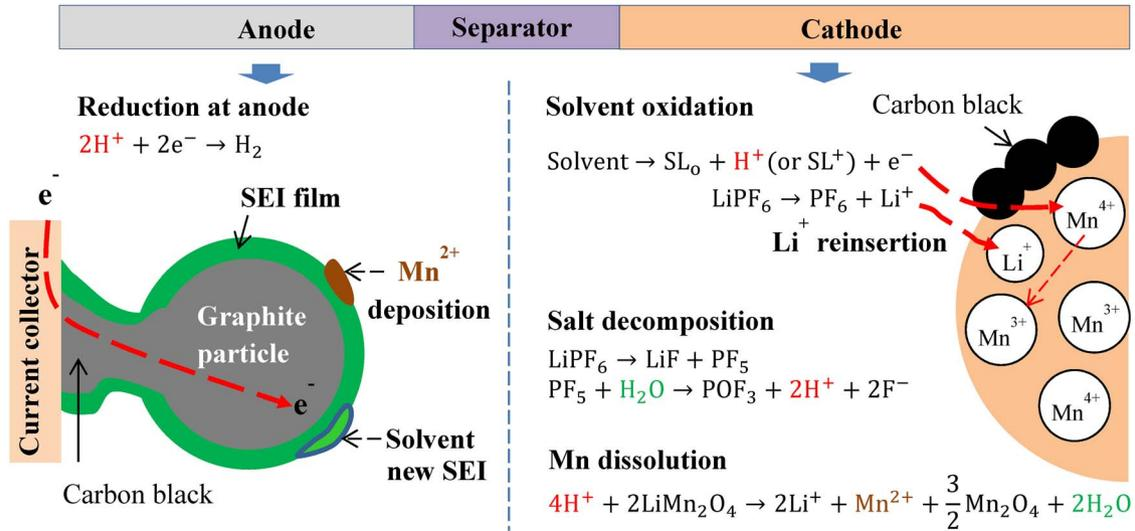
**Figure 1.** A schematic diagram of side reactions in the degradation model.
