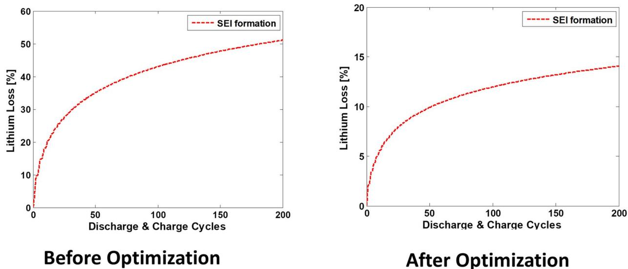
Figure 7. Cyclable lithium loss associated with SEI growth.
