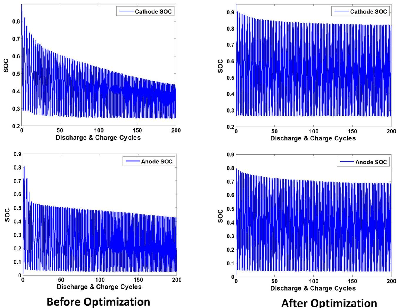
Figure 6. Comparison of the SOC swing window between a normal cell and the optimized cell.
