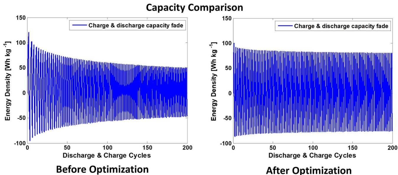
Figure 5. Comparison of capacity degradation between a normal cell and the optimized cell.
